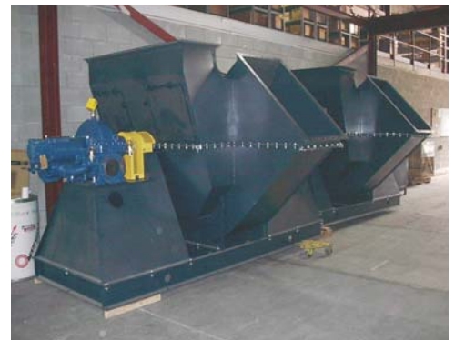
Dual drive combustion air fan
