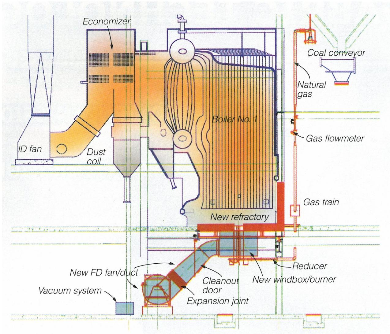
Lipten developed the vertical burner concept and has converted numerous boilers from coal to natural gas firing. Many facilities are upgrading their power plants by converting existing coal fired boilers to natural gas firing to:
